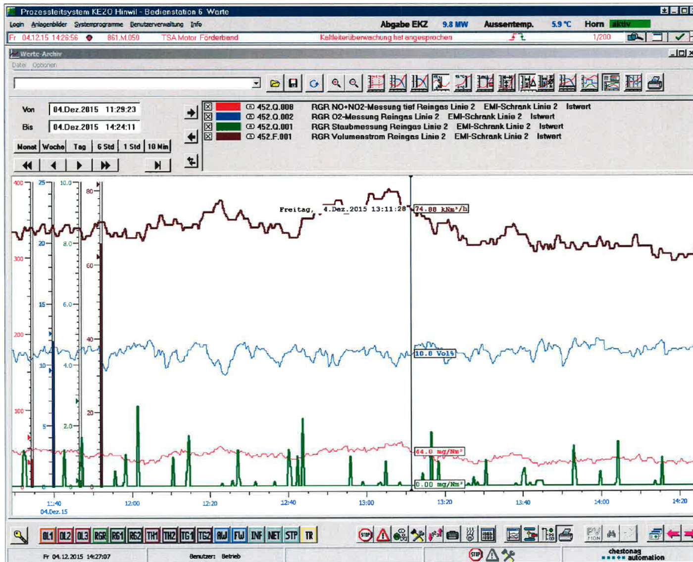
Figure A4. Time series of \text{NO}_x , \text{O}_2 , dust, and volume of air measured at Hinwil (ZH) on 12/4/2015 after the bag-house filter with probes belonging to the MSWI plant.
